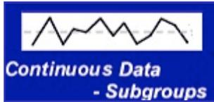
An **X-Bar and R-Chart** is a type of statistical process control chart for use with continuous data collected in subgroups at set time intervals - usually between 3 to 5 pieces per subgroup. The Mean (X-Bar) of each subgroup is charted on the top graph and the Range (R) of the subgroup is charted on the bottom graph. Out of Control points or patterns can occur on either the X-bar or R chart.
